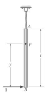
A thin rod having mass M is balanced vertically as shown. Determine the height h at which it can be struck with a horizontal force  $\mathbf{F}$  and not slip on the floor. This requires that the frictional force at A be essentially zero.
