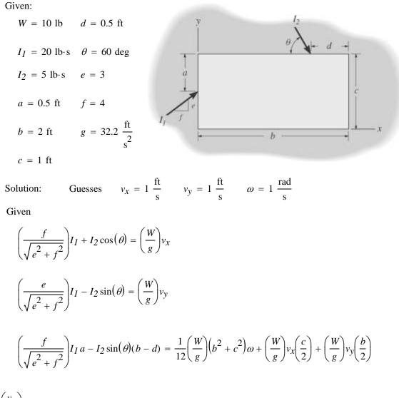
$$\begin{pmatrix} v_x \\ v_y \\ \omega \end{pmatrix} = \operatorname{Find}(v_x, v_y, \omega) \qquad \mathbf{v}_{\mathbf{G}} = \begin{pmatrix} v_x \\ v_y \end{pmatrix} \qquad \omega = -119 \frac{\operatorname{rad}}{\mathrm{s}} \qquad \mathbf{v}_{\mathbf{G}} = \begin{pmatrix} 59.6 \\ 24.7 \end{pmatrix} \frac{\mathrm{ft}}{\mathrm{s}}$$
