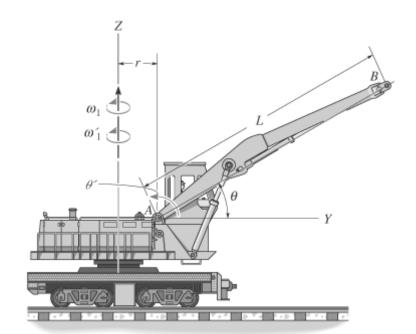
$$\mathbf{v_B} = \begin{pmatrix} 0 \\ v \\ 0 \end{pmatrix} + \begin{pmatrix} 0 \\ 0 \\ \omega_I \end{pmatrix} \times \begin{pmatrix} 0 \\ r \\ 0 \end{pmatrix} + \begin{pmatrix} \omega_2 \\ 0 \\ \omega_I \end{pmatrix} \times \begin{pmatrix} 0 \\ L\cos(\theta_I) \\ L\sin(\theta_I) \end{pmatrix}$$
