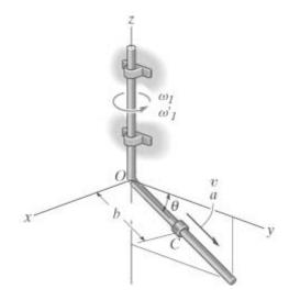
$$\mathbf{v_C} = v \begin{pmatrix} 0 \\ \cos(\theta) \\ -\sin(\theta) \end{pmatrix} + \begin{pmatrix} 0 \\ 0 \\ \omega_I \end{pmatrix} \times \begin{pmatrix} 0 \\ b\cos(\theta) \\ -b\sin(\theta) \end{pmatrix}$$
