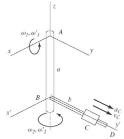
$$\mathbf{v_C} = \mathbf{v_B} + \begin{pmatrix} 0 \\ v_{CB} \\ 0 \end{pmatrix} + \begin{pmatrix} \omega_I \\ 0 \\ \omega_2 \end{pmatrix} \times \begin{pmatrix} 0 \\ b \\ 0 \end{pmatrix}$$
