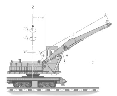
$$\mathbf{v_B} = \begin{pmatrix} 0 \\ 0 \\ \omega_I \end{pmatrix} \times \begin{pmatrix} 0 \\ r \\ 0 \end{pmatrix} + \begin{pmatrix} \omega_2 \\ 0 \\ \omega_I \end{pmatrix} \times \begin{pmatrix} 0 \\ L\cos(\theta_I) \\ L\sin(\theta_I) \end{pmatrix}$$
