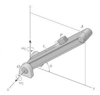
$$\mathbf{\omega} = \begin{pmatrix} \omega_{2} \\ 0 \\ \omega_{I} \end{pmatrix} \times \mathbf{\omega} \qquad \mathbf{rp} = \begin{pmatrix} 0 \\ r\cos(\theta) \\ r\sin(\theta) \end{pmatrix}$$
