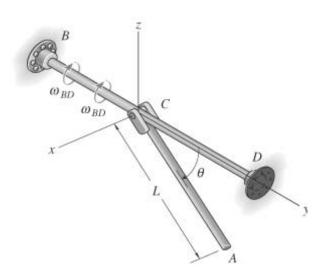
$$\mathbf{\omega} = \begin{pmatrix} -\omega_2 \\ -\omega_{BD} \\ 0 \end{pmatrix} \qquad \mathbf{\alpha} = \begin{pmatrix} -\alpha_2 \\ -\omega'_{BD} \\ 0 \end{pmatrix} + \begin{pmatrix} 0 \\ -\omega_{BD} \\ 0 \end{pmatrix} \times \mathbf{\omega} \qquad \mathbf{r_A} = \begin{pmatrix} 0 \\ L\cos(\theta_I) \\ -L\sin(\theta_I) \end{pmatrix}$$
