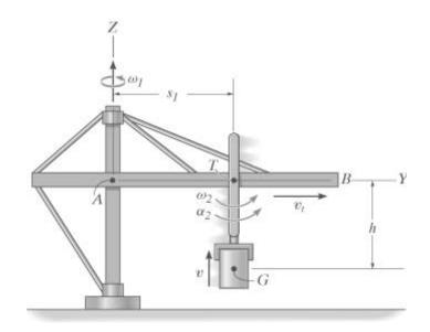
$$\mathbf{v_T} = \begin{pmatrix} 0 \\ v_t \\ 0 \end{pmatrix} + \begin{pmatrix} 0 \\ 0 \\ \omega_I \end{pmatrix} \times \begin{pmatrix} 0 \\ s_I \\ 0 \end{pmatrix}$$
