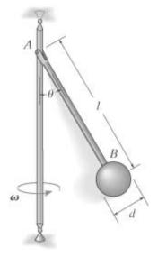
The rod *AB* supports the sphere of weight *W*. If the rod is pinned at *A* to the vertical shaft which is rotating with angular acceleration  $\alpha \mathbf{k}$ , and at the instant shown the shaft has an angular velocity  $\omega \mathbf{k}$ , determine the angle  $\theta$  of the rod during the motion. Neglect the mass of the rod in the calculation.
