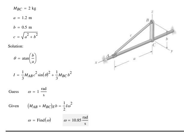
The rod has weight density  $\gamma$  and is suspended from parallel cords at *A* and *B*. If the rod has angular velocity  $\omega$  about the *z* axis at the instant shown, determine how high the center of the rod rises at the instant the rod momentarily stops swinging.
