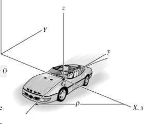
*Note*: This result indicates the normal reactions of the tires on the ground are not all necessarily equal. Instead, they depend upon the speed of the car, radius of curvature, and the products of inertia,  $I_{yz}$  and  $I_{zx}$ . (See Example 13-6.)
