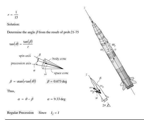
The projectile has a mass M and axial and transverse radii of gyration  $k_z$  and  $k_t$ , respectively. If it is spinning at  $\omega_s$  when it leaves the barrel of a gun, determine its angular momentum. Precession occurs about the Z axis.
