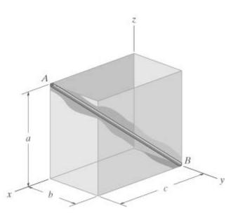
The bar of weight *W* rests along the smooth corners of an open box. At the instant shown, the box has a velocity  $v = v_I \mathbf{j}$  and an acceleration  $a = a_I \mathbf{j}$ . Determine the *x*, *y*, *z* components of force which the corners exert on the bar. Given:
