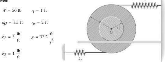
$$-k_{I}(r_{o}+r_{i})\theta(r_{o}+r_{i}) - k_{2}(r_{o}-r_{i})\theta(r_{o}-r_{i}) = \left(\frac{W}{g}k_{G}^{2} + \frac{W}{g}r_{i}^{2}\right)\theta'$$
