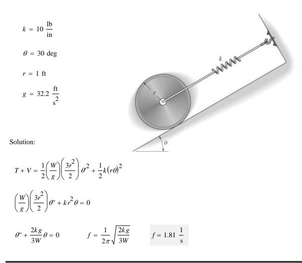
If the disk has mass M, determine the natural frequency of vibration. The springs are originally unstretched.
