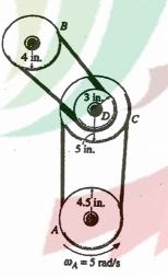
When  $\theta_{B} = 6 \text{ rev}$ ;  $4(6) = 3 \theta_{C}$   $\theta_{C} = 8 \text{ rev}$   $8(5) = 4.5(\theta_{A})$   $\theta_{A} = 8.889 \text{ rev}$   $(\omega_{A})_{2}^{2} = (\omega_{A})_{1}^{2} + 2\alpha_{C}[(\theta_{A})_{2} - (\theta_{A})_{1}]$   $(\omega_{A})_{2}^{2} = (5)^{2} + 2(2)[(8.889)(2\pi) - 0]$   $(\omega_{A})_{2} = 15.76 \text{ rad/s}$   $15.76(4.5) = 5\omega_{C}$   $\omega_{C} = 14.18 \text{ rad/s}$  $14.18(3) = 4(\omega_{B})_{2}$
