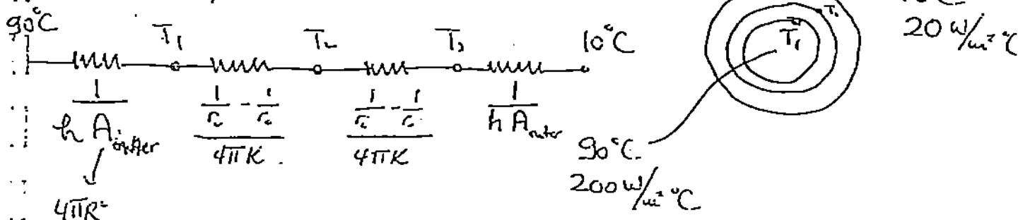
$q = \frac{\Delta T}{\Sigma R} = \frac{90-10}{\Sigma R} = 551.9 \text{ Watts}$
