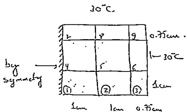
Node 1  $\frac{T_4 - T_1}{R_{14}} + \frac{T_2 - T_1}{R_{12}} + \dot{q} \Delta V = 0$        $R_{14} = \frac{0.01}{5 \times 0.01} ; \Delta V = 2.5 \times 10^{-5}$
