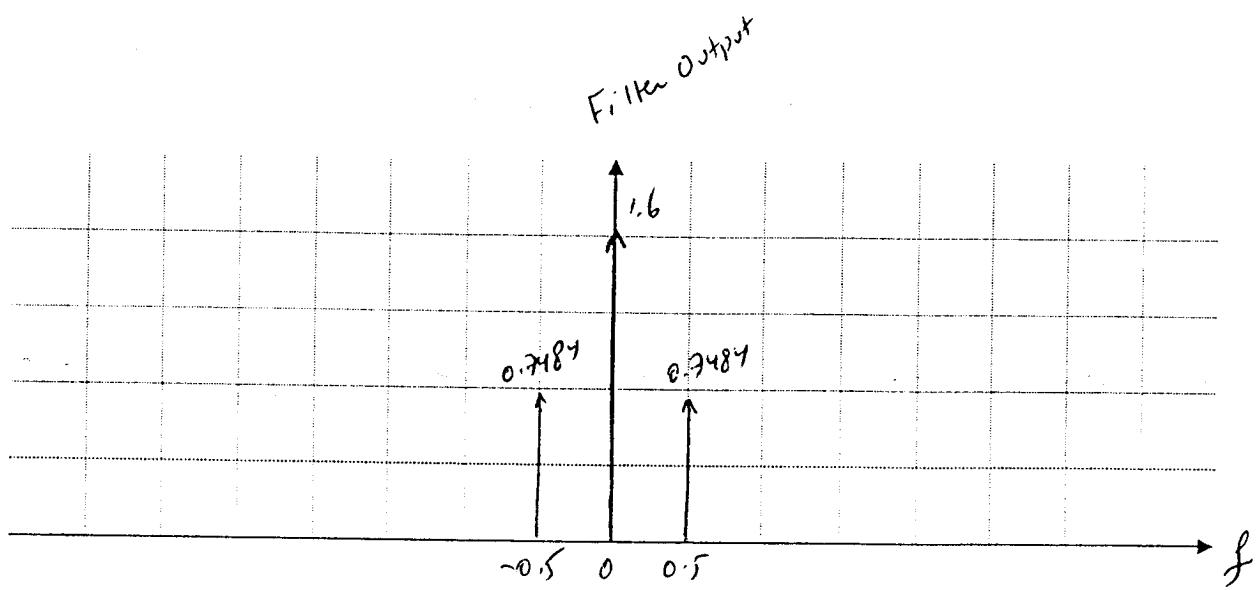
Output of filter:  $y(f) \rightarrow 3$  center delta functions
