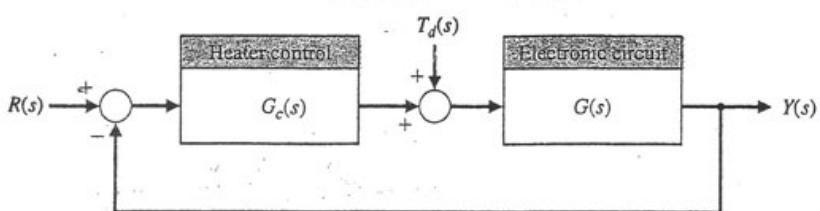
$$\begin{aligned} T.F. &= \frac{K}{s+10} \cdot \frac{2000}{s^2 + 6s + 5} = \frac{2000K}{(s+10)(s^2 + 6s + 5) + 2000K} \checkmark \\ &= \frac{1 + \frac{K}{s+10}}{1 + \frac{2000}{s^2 + 6s + 5}} \checkmark \\ &= \frac{2000K}{s^3 + 16s^2 + 65s + 50 + 2000K} \end{aligned}$$
