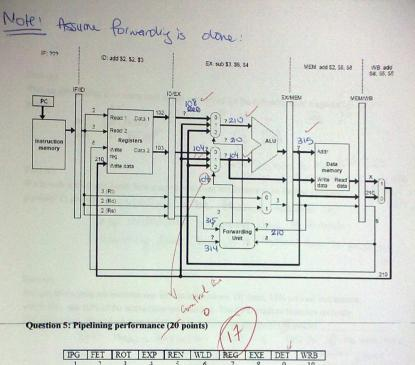
One CPU manufacturer has proposed the <u>10-stage pipeline</u> above for a <u>500MHz</u> (<u>2ns clock</u> cycle) machine. Here are the correspondences between this and the MIPS pipeline:
