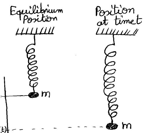
A mass  $m$  is attached to the lower end of a spring. If we push the mass  $m$   $y_0$  units and give it an initial velocity of  $v_0$  then  $m$  will oscillate about the equilibrium position.
