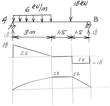
Beam AC is supported by a hinge at A and a roller at B. Draw shear and moment diagrams for AC using Method B; any other method will not count.
