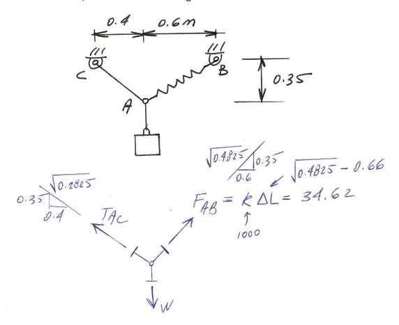
$$\frac{+}{\Rightarrow} = F_{x} = 0: \frac{0.4}{\sqrt{0.2825}} T_{AC} - \frac{0.6}{\sqrt{0.4825}} 34.62 = 0, T_{AC} = 39.736$$
