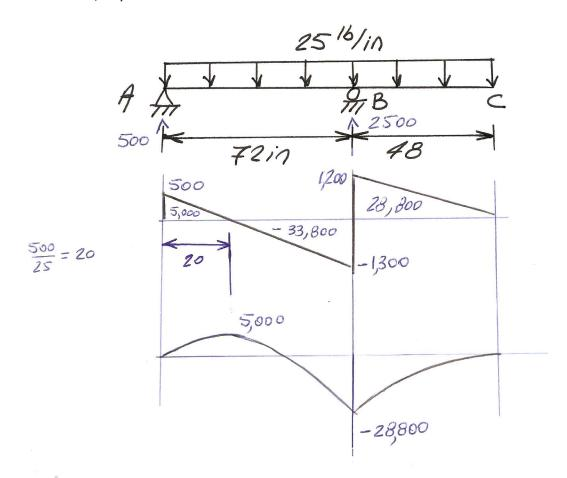
The shear and moment diagrams for beam AB are shown below. Determine and draw the loading that acts on the beam.
