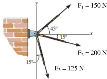
**Rectangular Components:** By referring to Fig.  $a$ , the  $x$  and  $y$  components of  $F_1$ ,  $F_2$ , and  $F_3$  can be written as
