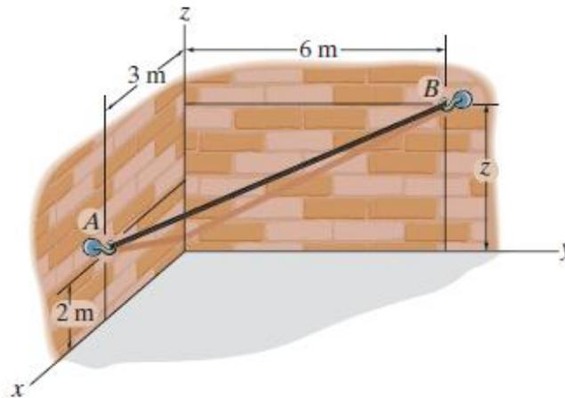
**Position Vector:** The coordinates for points  $A$  and  $B$  are  $A(3, 0, 2)$  m and  $B(0, 6, z)$  m, respectively. Thus,
