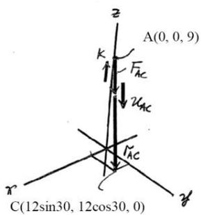
2-112. Determine the projected component of the force.  $F_{AB} = 560$  N acting along cable AC. Express the result as a Cartesian vector
