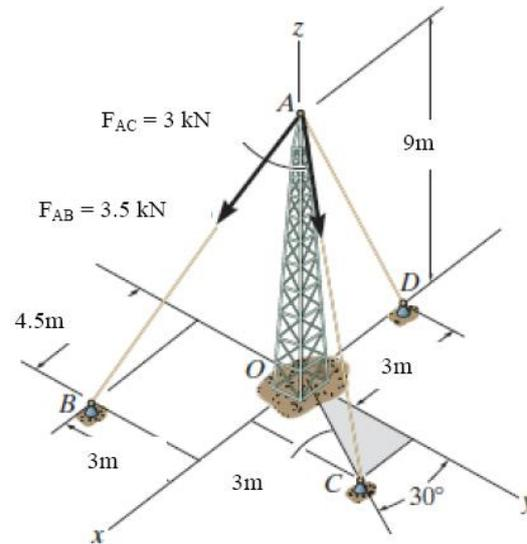
**Unit Vector:** The unit vector  $\mathbf{u}_{AC}$  must be determined first. From Fig. a,
