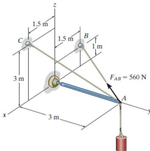
**Force Vectors:** The unit vectors  $\mathbf{u}_{AB}$  and  $\mathbf{u}_{AC}$  must be determined first. From Fig. a,
