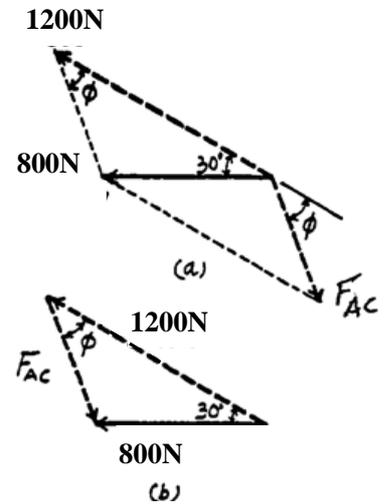
2–32. Determine the magnitude of the resultant force acting on the pin and its direction measured clockwise from the positive  $x$  axis.
