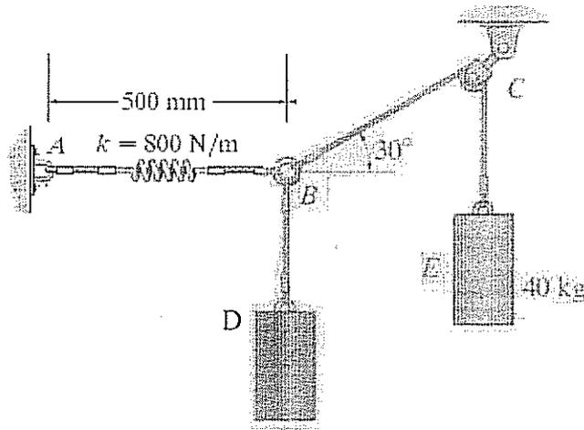
If the mass of cylinder  $E$  is  $40 \text{ kg}$ , determine the mass of cylinder  $D$  and the unstretched length of spring  $AB$ , in order to hold the assembly in the position shown. (30 points)
